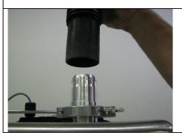
**NOTE:** If System was supplied with an over pressure relief device. Do not place the fume hood connection directly on the automatic pressure relief / exhaust valve. Place the connection over the valve as shown.
