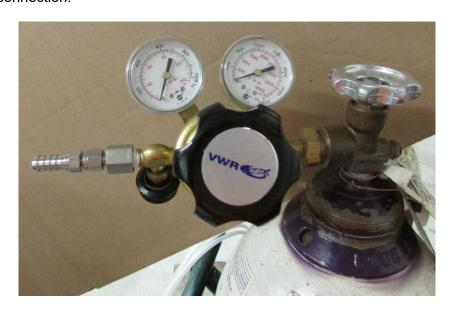
3. One (1) gas cylinder or gas source that is capable of delivering at least 200L/min flow rate of inert gas selected. This is a typical standard gas cylinder.
