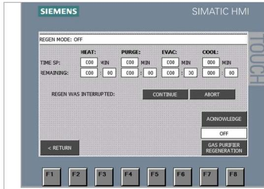
This screen shows that the regeneration has been interrupted due to the system being shut down during the regeneration cycle.
