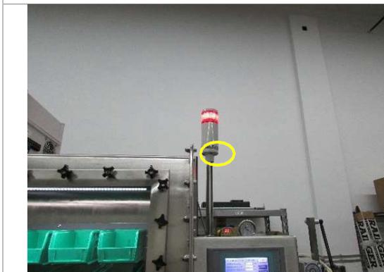
If the system was purchased with an alarm light and/or buzzer, the alarm/buzzer will trigger when the system is in an alarm state.
