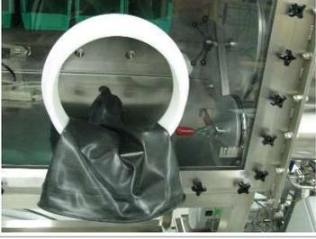
A black nitrile glove is being placed onto a circular white glove port on a stainless steel surface.                                     | <ol style="list-style-type: none"><li>1. Place the glove onto the glove port.</li></ol>                                                                                                                                                      |
