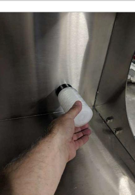
A close-up photograph showing the same hand from the previous image, now pushing the white filter into the stainless steel base. The filter is partially inserted into a circular opening in the metal. The hand is positioned to apply pressure to the side of the filter.                        | <ol style="list-style-type: none"><li>2. Push filter until it is flush with base.</li></ol> |
