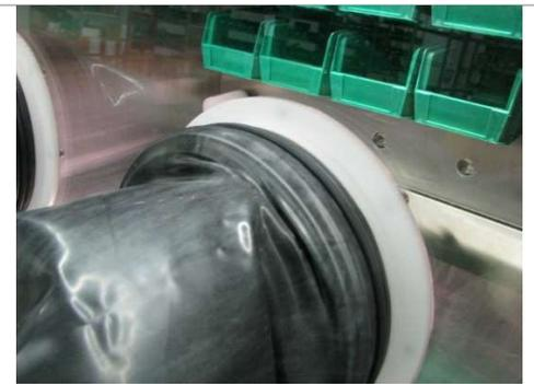
6. Reach into the new glove and carefully grab folded back edge of the old glove.
