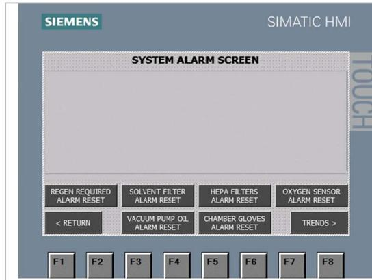
This alarm indicates that it is recommended to run a regeneration at this time. The filter column on your system is most likely reaching capacity and will need to be regenerated soon.
