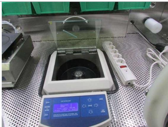
2. Place substrate on spin coater chuck.
