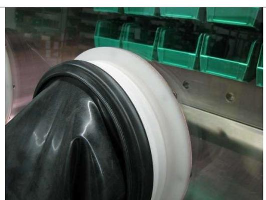
A close-up photograph showing the black glove being folded back over the white component. The O-ring is now visible, having been repositioned under the folded edge of the glove. The background is consistent with the previous images. | <p>3. Fold the glove back over the existing O-ring.</p> |
