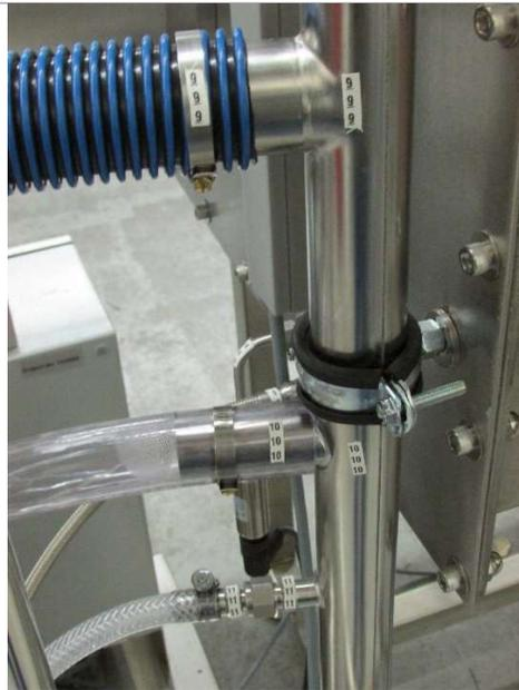
Various components of the glovebox will need to be attached to the system. These components have been labeled to show connection points. Match corresponding numbers (i.e. 1 to 1; 2 to 2; and so on).
