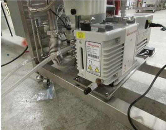
A photograph of an Edwards vacuum pump unit, which is a white rectangular device with a black cap on top, mounted on a metal base. It is connected to various hoses and pipes. | <p>2. Remove the black cap at the end of the drain. Place a container under the drain to capture the oil.</p>                                                                      |
