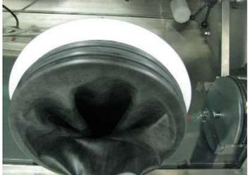
A second white O-ring is being placed into the outermost groove of the black nitrile glove, which is attached to the white glove port. | <ol style="list-style-type: none"><li>5. Place the second glove O-ring in the outermost glove port groove.</li></ol>                                                                                                                         |
