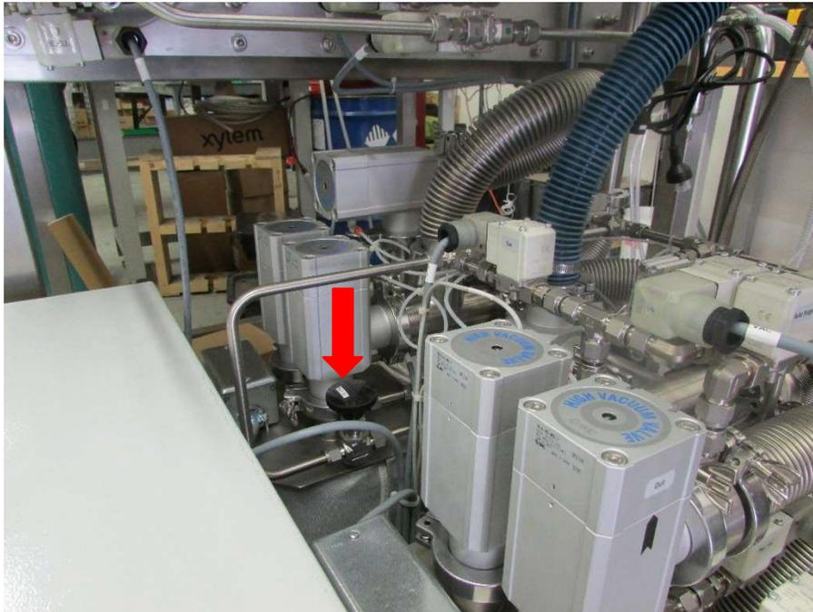
Newer models will have a regulator and flow meter (pictured below on the left). The regulator will come factory set at 20 psi and the flowmeter will also come factory set for 15 l/min. The flow meter will not display its flow rate until the reactivation phase. (Pictured below on the right).
