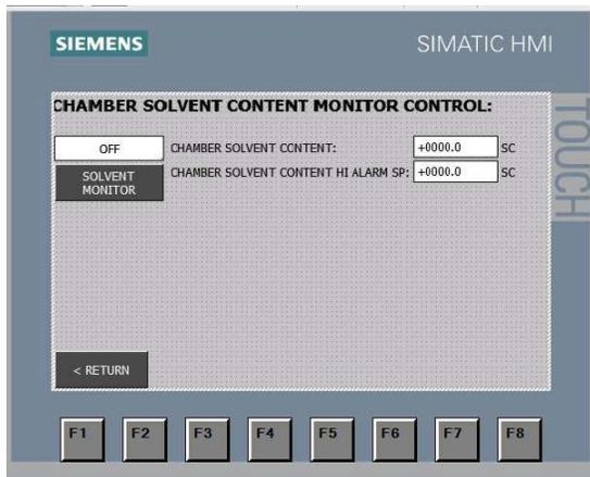
By pressing the button on the main screen that says Solvent Monitor you will see the screen to the left. It displays the current solvent content inside the glovebox. It also displays the user adjustable set point for the solvent sensor alarm. This is typically set to 0.1 as you will want to get an alarm as soon as there is excess solvent vapor inside the glovebox.
