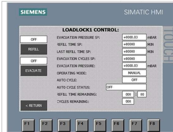
4. Evacuation Cycles SP – this allows the user to set the number of EVAC/Refill cycles the chamber will perform.
