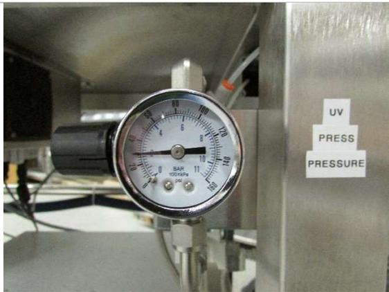
11. Verify UV press clamping pressure is set at 30 psi.
