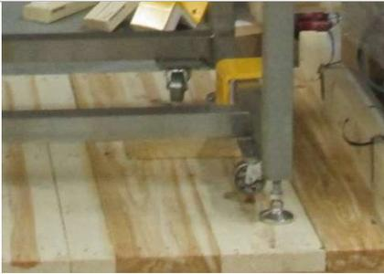
2. Lower the stand onto its wheels by adjusting the leveling feet with a wrench.
