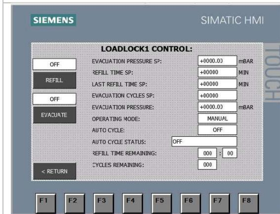
5. To begin automatic antechamber control, change the Evacuation Cycles SP to 3 by pressing the white button to the right.
