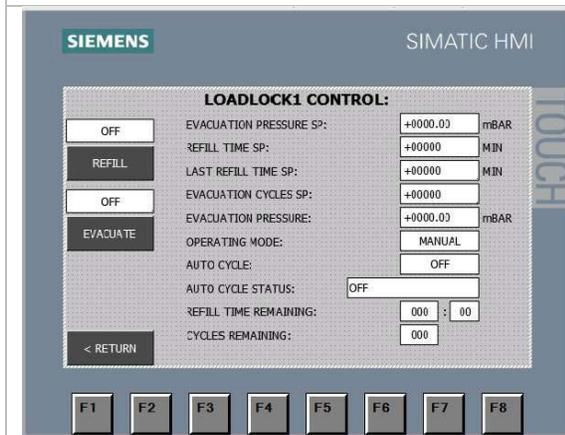
3. Last Refill Time SP = this set point is the final refill cycle and should be longer than the second refill time.
