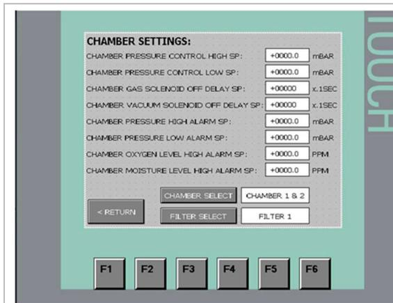
1. For systems supplied with 2 filter columns, you will need to select the active filter column. The activated filter column is the column that you wish to use to circulate the glovebox environment. The other column will be in standby mode.
