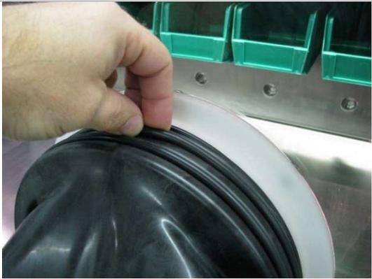
A close-up photograph showing a person's hand pulling a black O-ring away from the edge of a black glove. The glove is mounted on a white cylindrical component. In the background, there are green plastic trays on a metal surface.      | <p>1. Remove the O-ring nearest to the window.</p>      |
