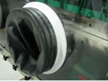
A hand is shown inside the black nitrile glove, which is now attached to the white glove port.                                           | <ol style="list-style-type: none"><li>2. Place your hand in the glove and align the glove in a comfortable position, with thumbs facing upwards.</li><li>3. Move the glove forward until it meets the innermost glove port groove.</li></ol> |
