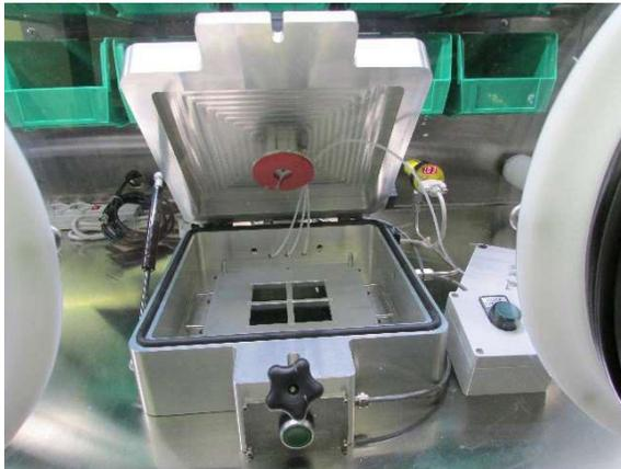
3. Load substrate into substrate holder.
