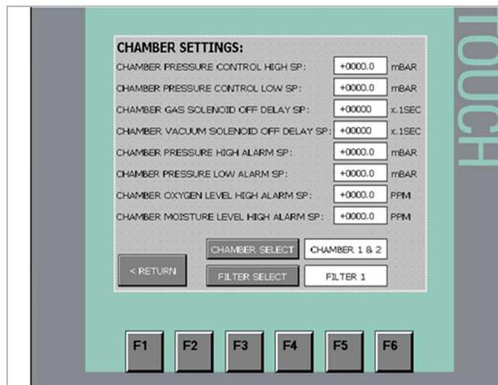
If your system was configured with dual filter columns, you can circulate your system and regenerate the other filter column at the same time. The system automatically regenerates the filter column that is not being used for circulation mode. In the chamber settings menu, filter 1 is selected for circulation therefore filter 2 will be regenerated. Please follow the instruction in Section 15.1 to regenerate your filter column.
