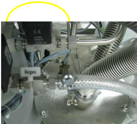
2. Find the tube labeled Regas and connect this tube to your regeneration gas supply.
