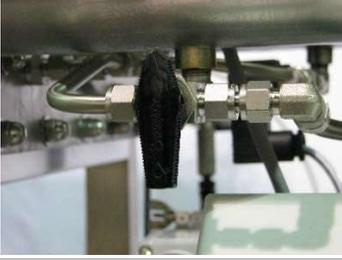
A photograph showing a close-up of a hand valve on a piece of industrial equipment. The valve handle is in the up position, indicating it is closed. | <p>11. Return hand valve to up (closed) position.</p>                                                                                                                                                                                                                                   |
