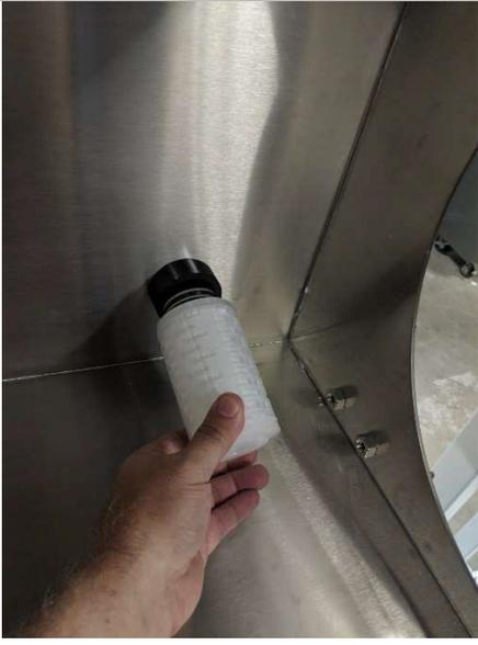
A close-up photograph showing a person's hand holding a white, cylindrical filter with a black top. The filter is being held against a curved, stainless steel surface, which is the base of the equipment. The background is slightly out of focus, showing more of the stainless steel structure. | <ol style="list-style-type: none"><li>1. Take new filter and align to base.</li></ol>       |
