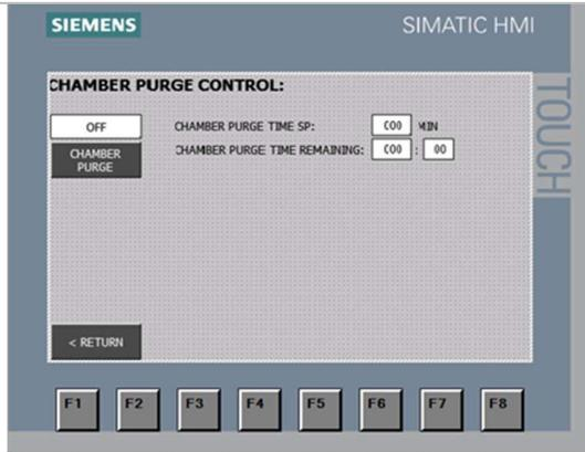
6. Chamber Purge Time Remaining reflects the amount of time remaining in the purge cycle.
