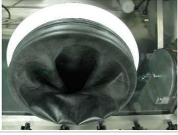
A white O-ring is being placed into the center groove of the black nitrile glove, which is attached to the white glove port.            | <ol style="list-style-type: none"><li>4. Place the first glove O-ring in the center glove port groove.</li></ol>                                                                                                                             |
