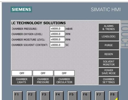
When the oxygen level reaches the alarm set point the system turns OFF circulation and starts to purge the system. The purge button will turn **green** when purging is happening.
