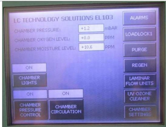
1. From Main Screen press Laminar Flow Units button.
