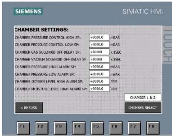
This option allows the user to set the automatic purge function to the alarm levels of the oxygen and moisture inside the glovebox. Most customers use this to automatically purge the glovebox if the oxygen level exceeds the alarm.
