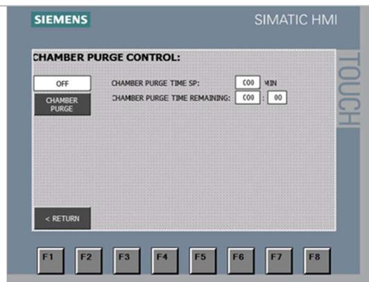
When the alarm is triggered, the automatic purge will activate and run for the amount of time set on the Chamber Purge Control screen. It will continue to purge even after the alarm has cleared for the time set in this function screen.
