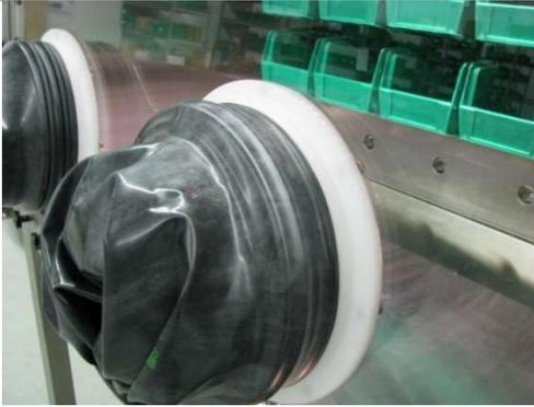
4. Place new glove over the old glove. Make sure the new glove is mounted in the O-ring groove.
