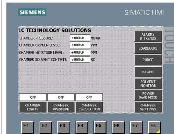
Press Chamber Pressure Control to enable pressure control and glovebox circulation.
