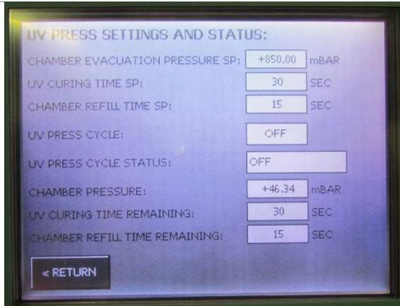
10. Set desired set point by pushing white box to the right of set point.
