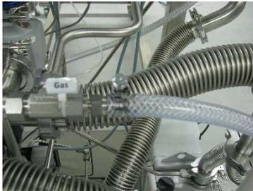
1. Find the tube labeled Gas and connect this tube to your inert gas (nitrogen or argon) supply
