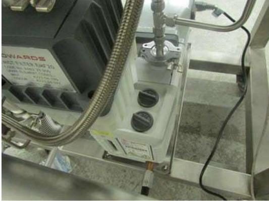
A close-up photograph of the Edwards vacuum pump unit, showing the oil fill plugs and the drain port. The pump is white and has a black cap on top.                           | <p>3. Remove one of the oil fill plugs.</p>                                                                                                                                        |
