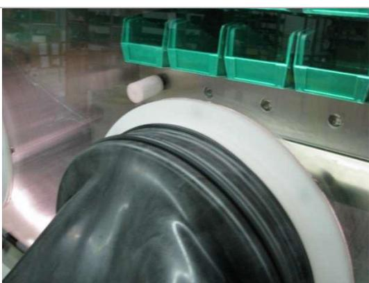
A close-up photograph of the black glove on the white component. The O-ring has been removed, and the glove is slightly lifted from the component. The background shows the same green trays and metal surface.                           | <p>2. Glove with O-ring removed</p>                     |
