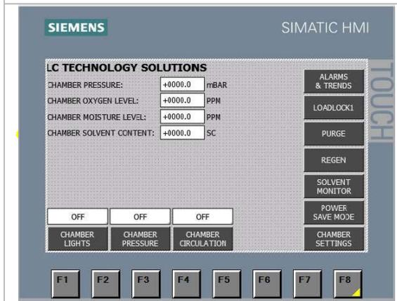
If you purchased an optional Solvent Sensor, this screen would provide the content of vapor inside the chamber.
