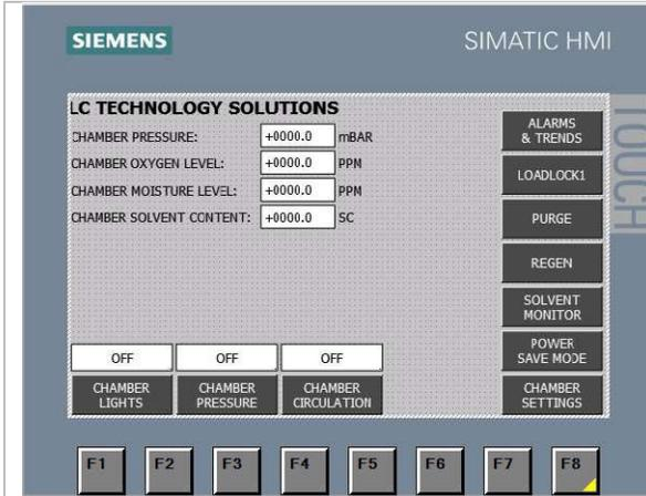
The power saver mode is designed to switch off the vacuum pump and/or lights when they are not needed to run the system. This saves both energy and cuts down on noise.
