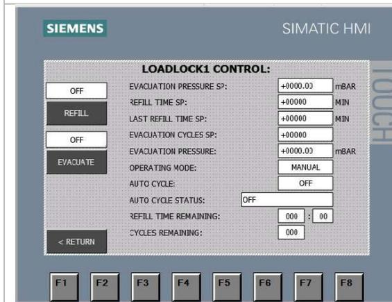
2. Refill Time SP – this is the length of time the chamber will refill before another evacuation cycle is started.
