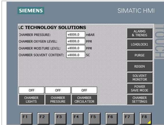
The main screen provides the current PPM level of oxygen and moisture inside the chamber.
