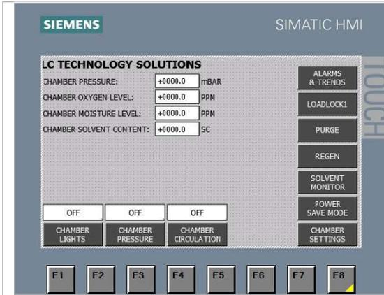
When the purge time has elapsed, the system will automatically turn circulation ON, **On** will be displayed and it will turn **Green** and purge will now be OFF.
