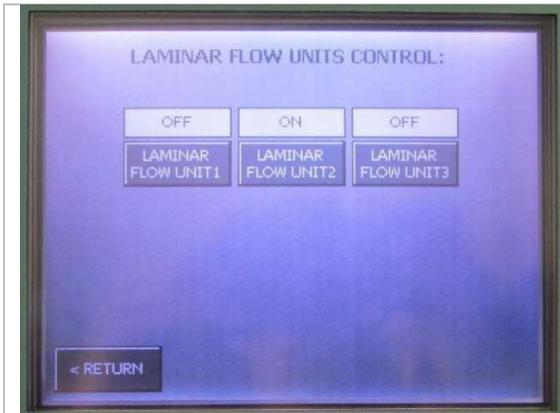
3. Push Laminar Flow Unit button to turn laminar flow ON or OFF.
