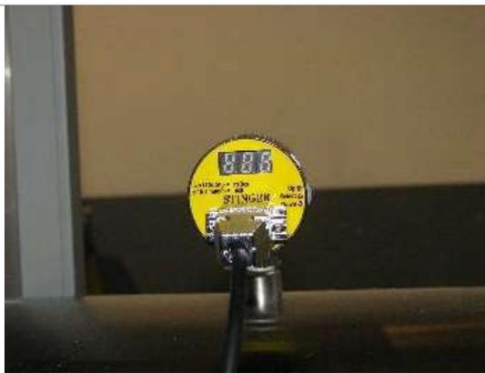
The vacuum level is shown on the gauge mounted on the top of the antechamber and on the PLC screen.
