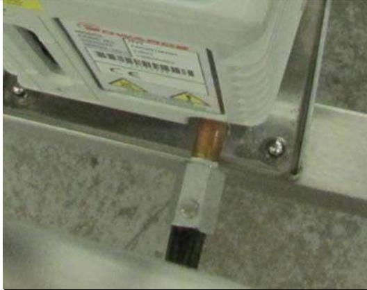
4. To open the drain valve, use a flat head screwdriver and turn the screw. The oil will start to flow out of the vacuum pump. When it is empty, return the screw to the closed position.
