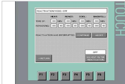
After 9 hours the Reactivation Cycle will be complete the system will say **COMPLETE**,
