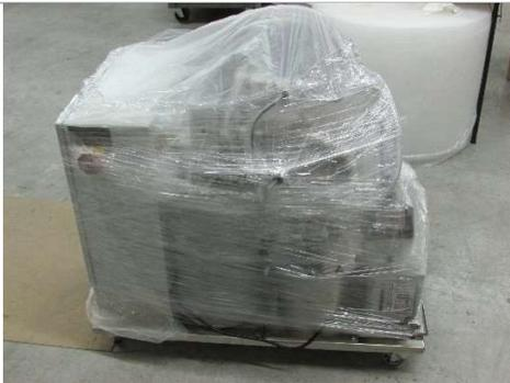
3. Remove purifier from crate. Use a forklift to remove from pallet, if available.
