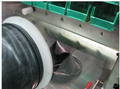
7. Pull the folded back edge of the old glove until the old glove and O-ring fall into the glovebox.
