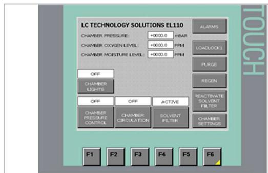
At the Main Menu put the system back in Active Mode by pressing the Solvent Filter button. **ACTIVE** should be displayed.
