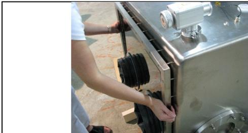
3. Remove the window frame and set aside.
