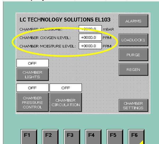
The main screen provides the current PPM level of oxygen and moisture inside the chamber.
