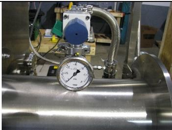
7. Close evacuation valve by turning the evacuation hand valve to the right.
