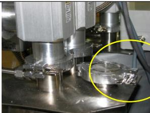
5. Replace KF40 cover and clamp on top of solvent filter.
