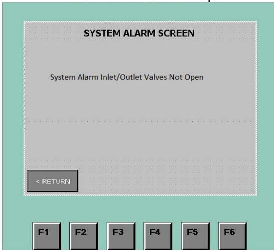
This alarm means that the electro-pneumatic valves on top of the filter column are not opening properly.
