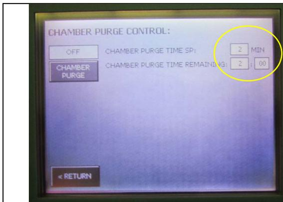
When the alarm is triggered the automatic purge will activate and run for the amount of time set on the Chamber Purge Control screen. It will continue to purge even after the alarm has cleared for the time set in this function screen.
