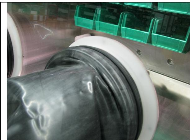
6. Reach into new glove and carefully grab folded back edge of old glove.
