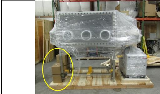
1. Cut banding straps and remove boxes containing loose parts for glovebox system.
