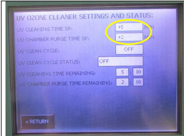
5. Set desired cleaning and purging time by pressing the white box to right of set point.
