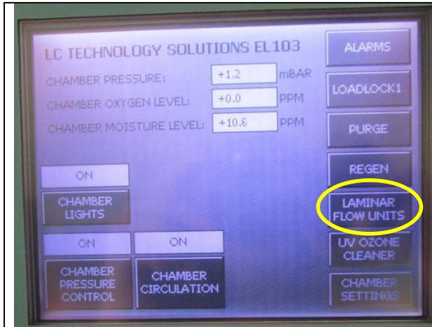
1. From Main Screen press Laminar Flow Units button.
