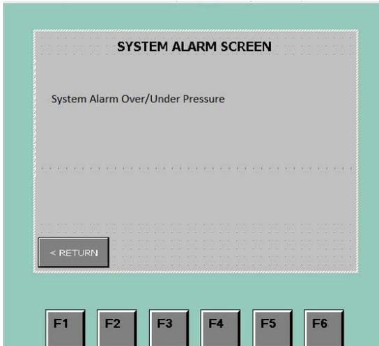
The Low Pressure Alarm means the system is under-pressurized. Once the glovebox goes above the low pressure safety set point it will shut off.
