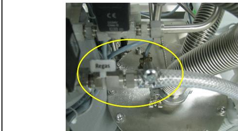
2. Find the tube labeled Regas and connect this tube to your regeneration gas supply.
