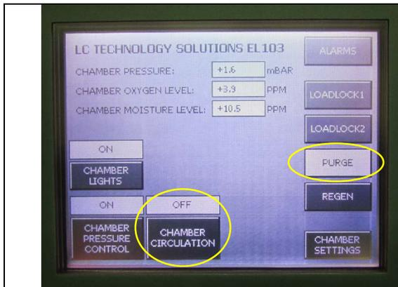
When the oxygen level reaches the alarm set point the system turns off the circulation and starts to purge the system.
