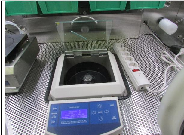
2. Place substrate on spin coater chuck.
