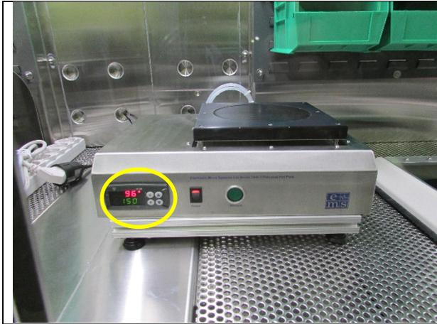
4. To adjust the temperature press and hold down the down arrow key.
