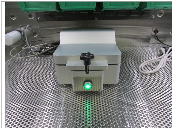
6. Press green button on front of UV ozone cleaner to start process. Button will illuminate.
