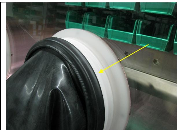
3. Fold glove back over existing O-ring as shown to the left.
