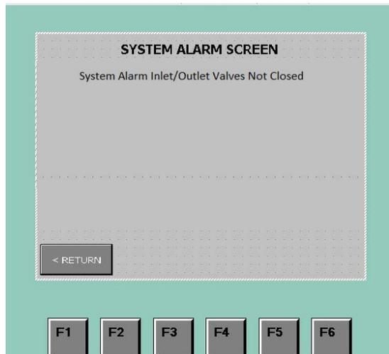
This means the valves on top of the filter column are not closed and you will be unable to perform the regeneration.
