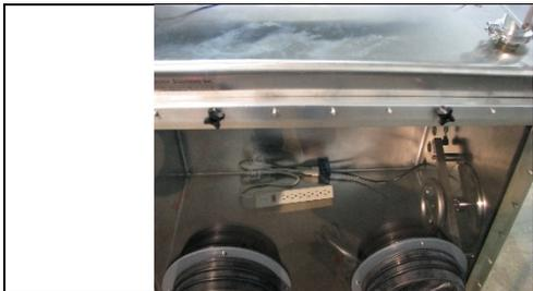
2. Remove the remaining star knobs being careful not to let the window and window frame fall.
