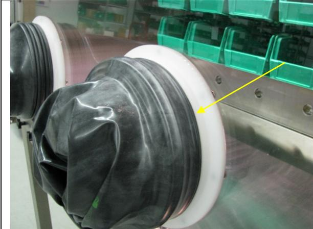
4. Place new glove over the old glove. Make sure the new glove is mounted in O-ring groove.
