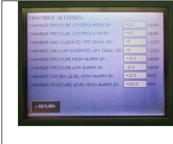
This option allows the user to set the automatic purge function to the alarm levels of the oxygen and moisture inside the glovebox. Most customers use this to automatically purge the glovebox if the oxygen level exceeds the alarm.
