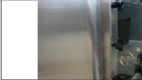
5. Tighten star knobs until window frame contacts glovebox.
