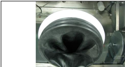
5. Place second glove O-ring in outer most glove port groove.
