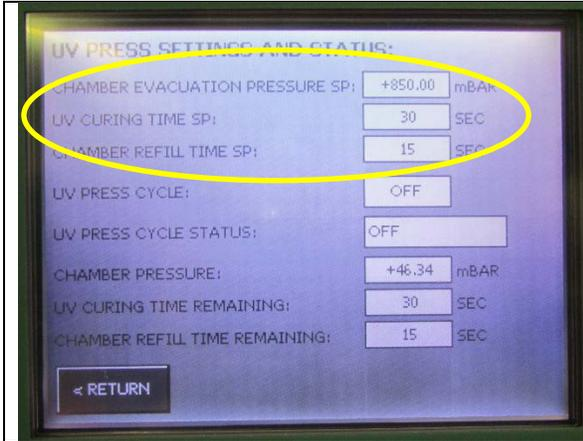
10. Set desired set point by pushing white box to the right of set point.
