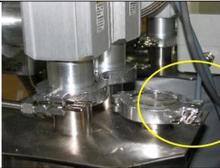
2. Remove KF40 clamp and cover on the fill/empty port on top of solvent removal system.
