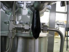
6. Using Valve 4 mounted on the back of the system evacuate the solvent removal system for approximately 24 hrs by turning Valve 4 to the left. The valve should be pointing towards the line that goes to the vacuum pump.
