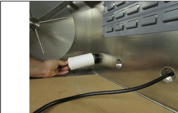
3. Replace old filter with the new one by pushing it into place in the socket.
