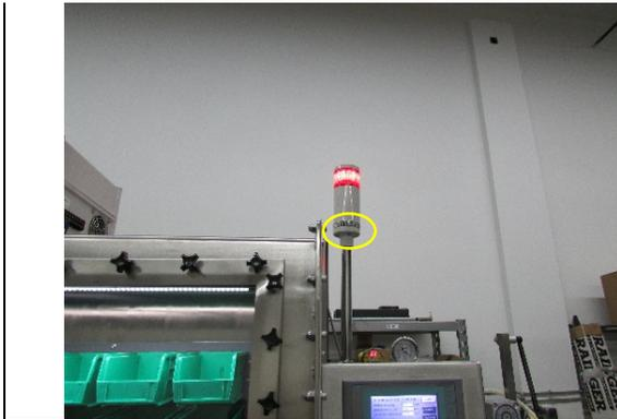
If the system was purchased with an alarm light and/or buzzer, the alarm/buzzer will trigger when the system is in an alarm state.
