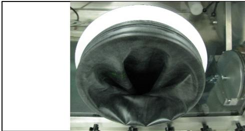
4. Place first glove O-ring in center glove port groove.
