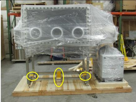
1. Once sides are off, unbolt lag bolts from Z-brackets using a  $\frac{3}{4}$ " wrench.
