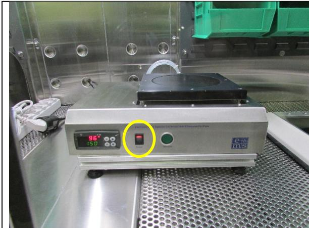
2. Turn power on by pushing switch down.
