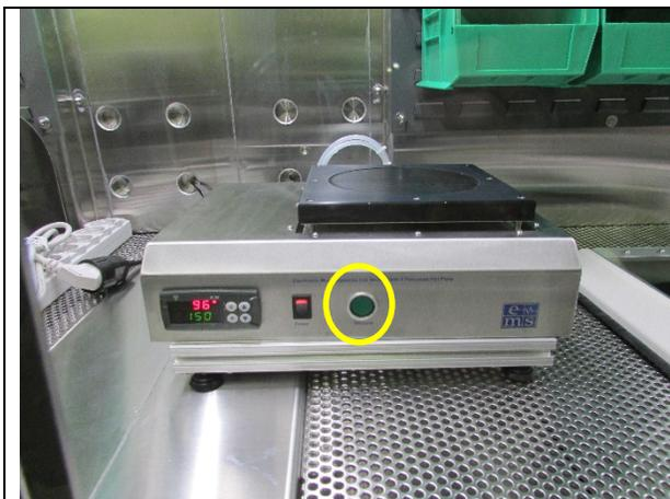
3. Press vacuum button to vacuum substrate down.
