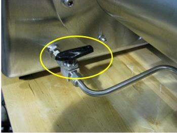
8. For glovebox models with manual refill, refill antechamber using Swagelok refill valve.
