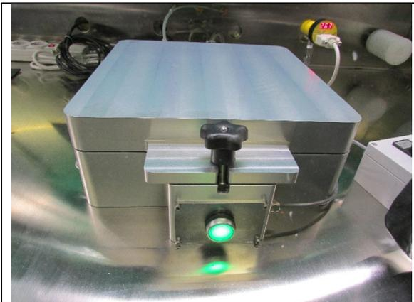
12. Press green button on front of UV press to start process.
