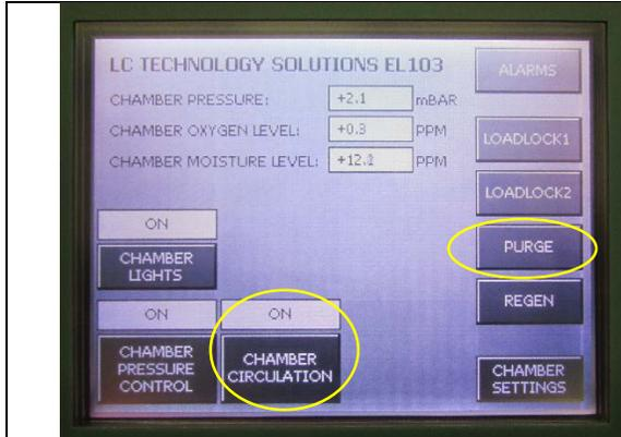
When the purge time has elapsed the system will automatically turn circulation on and purge off.
