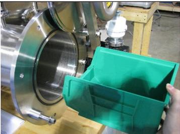
3. Place green bin inside antechamber; bin should be loaded into chamber short side first.
