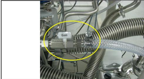
1. Find the tube labeled Gas and connect this tube to your inert gas (nitrogen or argon) supply.
