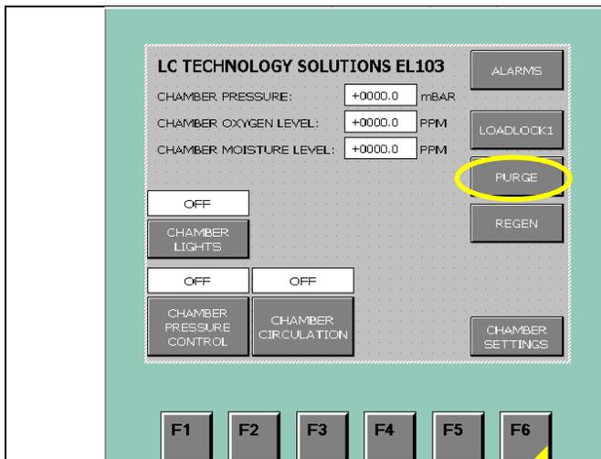
The screenshot shows the same control interface as above. The 'PURGE' button is now highlighted with a yellow circle. The 'CHAMBER CIRCULATION' button is no longer highlighted.
