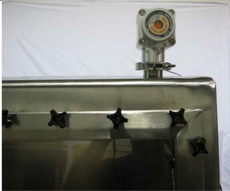
3. Open manual purge valve until you hear gas inlet valve come on and stay on.
