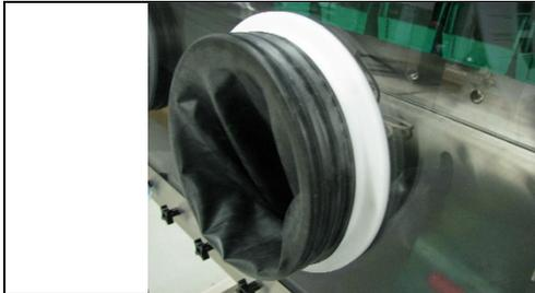
2. Place hand in glove and align glove hand in a comfortable position with thumbs facing in an upward position.
