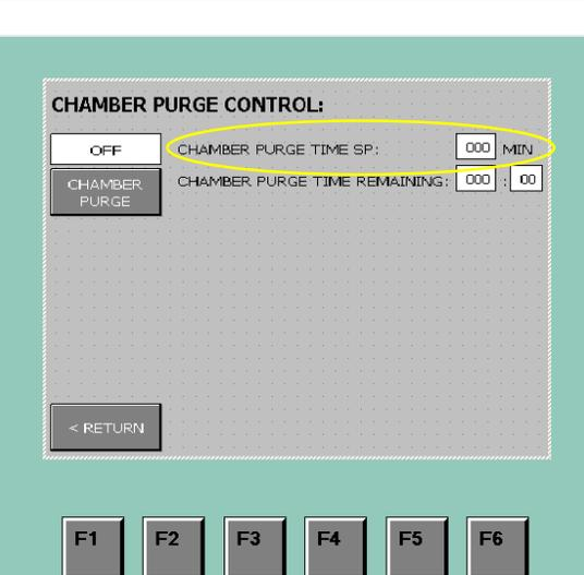
The screenshot shows the 'CHAMBER PURGE CONTROL' interface. At the top left, there is a white button labeled 'OFF' and a grey button labeled 'CHAMBER PURGE'. To the right, there are two digital displays: 'CHAMBER PURGE TIME SP:' showing '000 MIN' and 'CHAMBER PURGE TIME REMAINING:' showing '000 : 00'. A '< RETURN' button is located at the bottom left of the screen. Below the screen are six function keys labeled F1 through F6.
