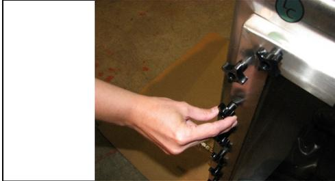
1. Undo all star knobs with the exception of two (2) at the top and two (2) at the bottom.
