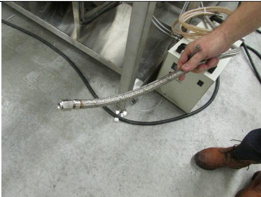
**NOTE:** Liquid nitrogen must be connected to the liquid nitrogen feed line for the plate to cool.
