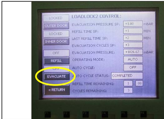
6. Push Evacuate button. This will allow it to run for 3 cycles.
