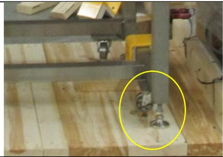
2. Lower stand onto its wheels by adjusting leveling feet with wrench.
