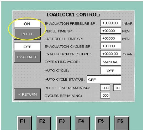
9. Repeat the above cycle two (2) more times for a total of three (3) evacuation/refill cycles.
