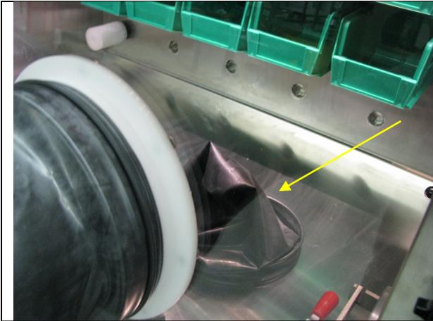
7. Pull folded back edge of old glove until the old glove and O-ring fall into the glovebox.
